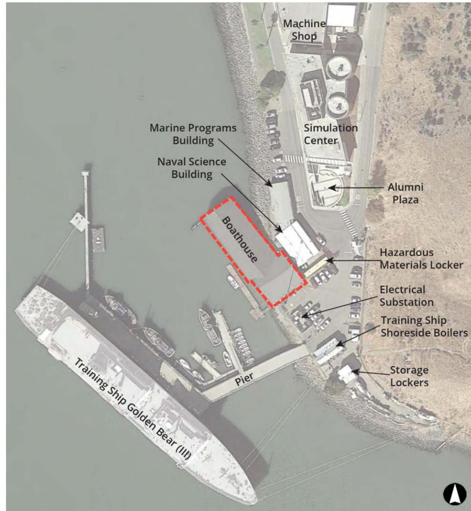
Figure 26: Buildings and structures located around the Boathouse (outlined with dashed red line). Source: Page & Turnbull. Base map: Google Earth aerial photograph, 2021.
