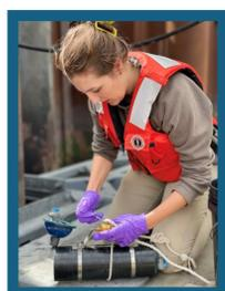
3) **Discrete Water Sampling** Water was collected by Van Dorn bottle within 1 m of surface. 150-200mL water was filtered onto 47mm GF/F for analysis.
