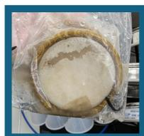
2) **Solid Phase Adsorption Toxin-Tracking (SPATT)** Samplers were deployed for 48 h and 2 to 4 weeks. SPATT was frozen until analysis
