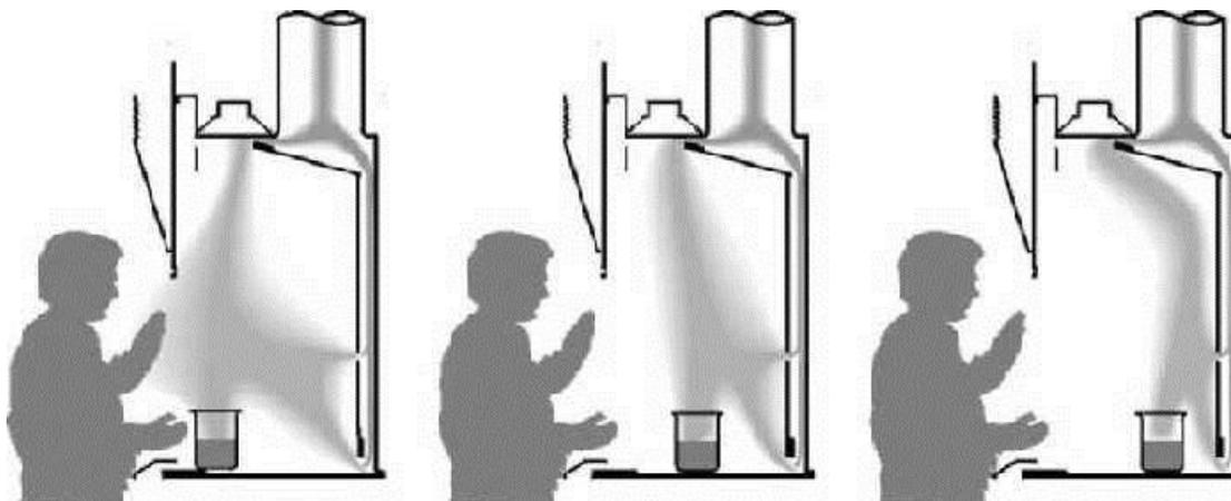
**Figure 2:** Containment of vapors in a chemical fume hood as a function of working distance.
